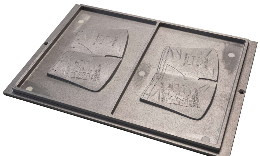
Completed Metapor-plate for the deep drawing.
